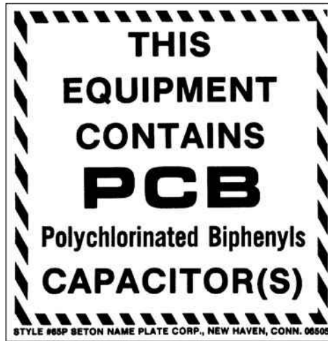
Figure 24.8 Marking label (ML) used to identify PCB transformers and PCB large capacitors.
