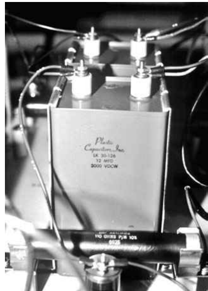
Figure 5.5 An oil-filled, high-voltage capacitor.
